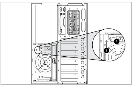
Figure 4-9. Power supply LEDs
